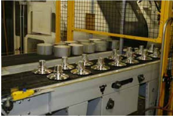
Fully automated machining center, the blanks go on one belt and the finish parts come out on the other.
