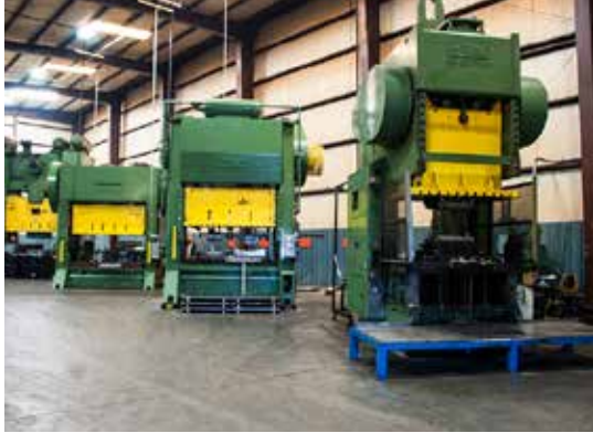
Superior Metal Products' 40+ hydraulic, pneumatic, and mechanical presses and press brakes range in tonnage from 10 to 600 tons.
