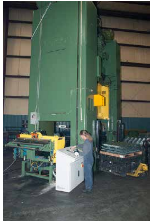
600-ton Verson stamping press with 48" x 108" bed at Superior Metal Products.
