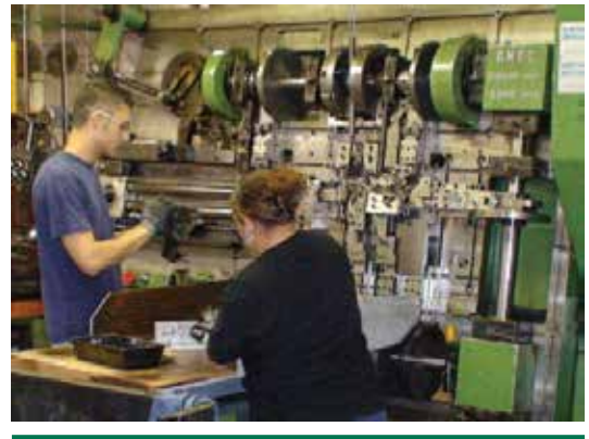
A series of multi-slide metal strip processors produce high quality mounting plates for automobiles and ATVs.
