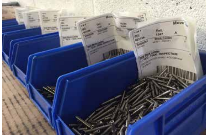
Move tickets identify where the parts have come from and where they are going for the next operation.
