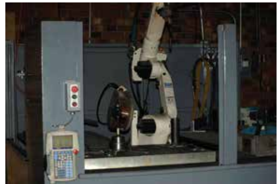
P&S Machining and Fabrication's four-station robotic welder for precision production welding
