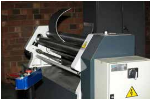
A P&S Machining and Fabrication's machine bending a metal part.
