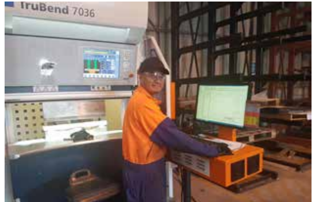
Metalform's pressbrake operator Chris Hulegas using a Shop Floor Data Collection station. Online drawings enable a paperless shop floor.
