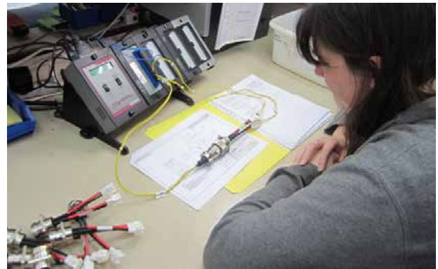
An employee testing cables at the MRG testing center.
