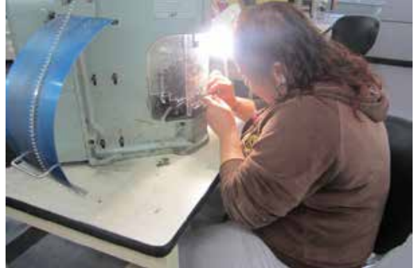
A worker machine crimping at MRG.
