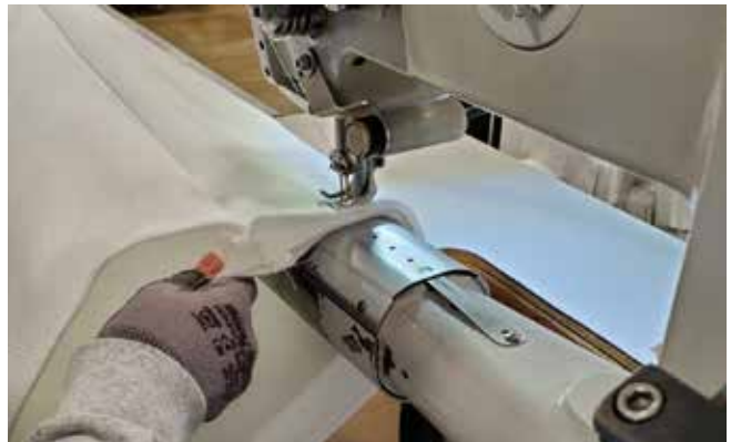
IFM's filter bags are made from high-quality polyester and polypropylene.
