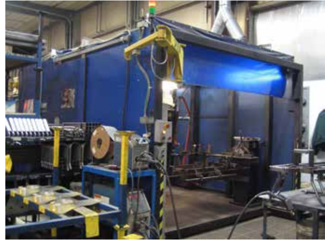
Fixturing for complicated welding jobs is aided by the use of welding fixture tables.
