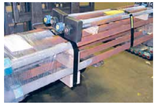
Recently completed double-ended studs with anchor plates.
