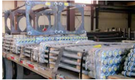
Hook anchor bolts and 18J rebar cages ready for shipment.
