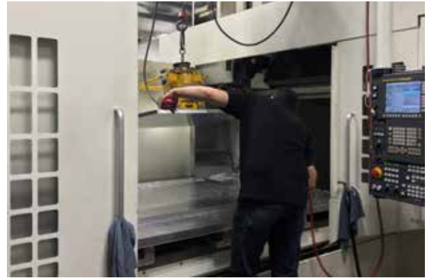
An operator is taking off a part mid-production to check for flatness before continuing to machine.
