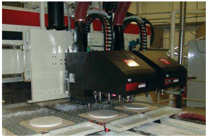
EPTAM’s capabilities include three high-speed CNC routers designed to efficiently produce precision components from large sheet stock.
