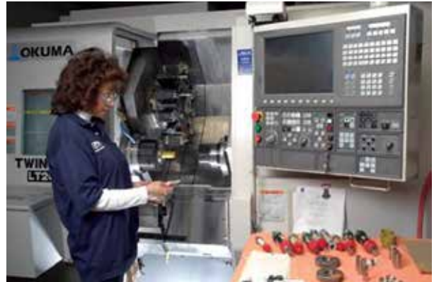
In lathe cell area, an operator prepares her machine for live-tooling for precision machining according to work orders routed through EPTAM's Shop Floor Data Collection system.
