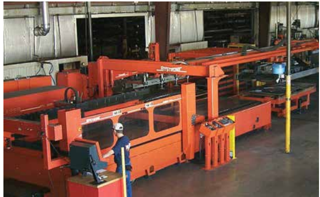
One of DeJong's fully-automated CNC laser cutting cells.
