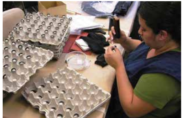
CGR hand-assembles their custom manufactured rubber O-rings to the inside of client supplied metal O-rings.
