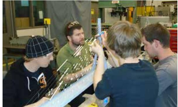
*Team members are building a 16-foot full aero elastic bridge model. This bridge was constructed in Spain.*
